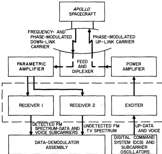
Fig. 3. Two-way communication function
