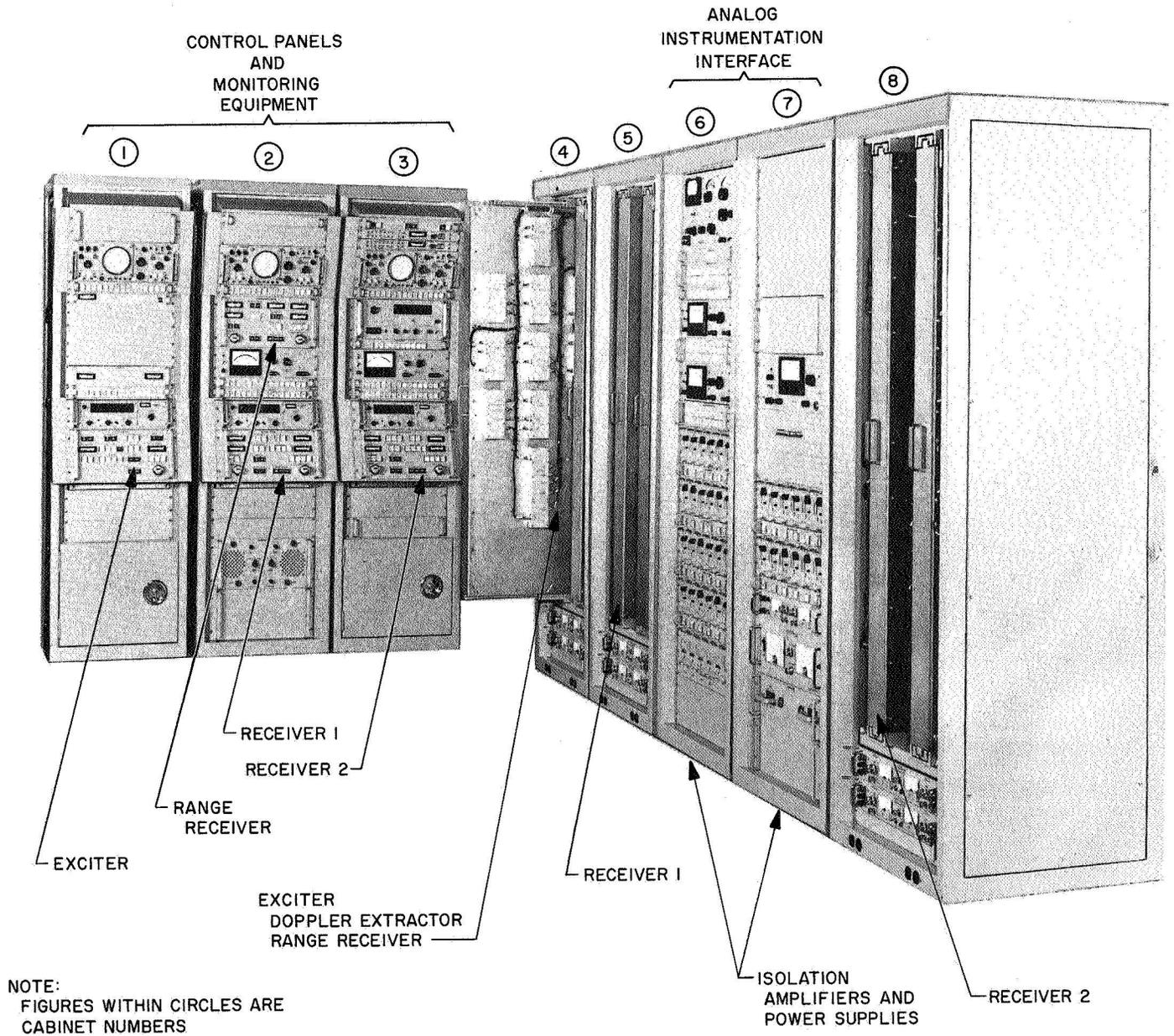
**Fig. 9. Receiver-exciter subsystem components and functions**
