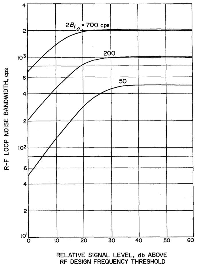
Fig. 7. Effect of variation in loop noise bandwidth on relative signal level
