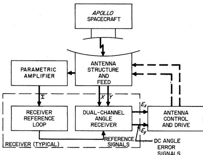
Fig. 4. Angle-tracking function
